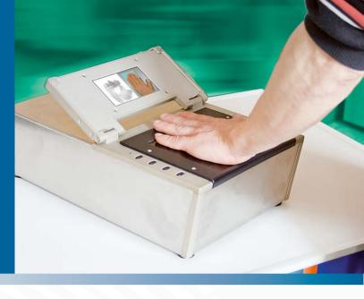
PAPILLON's optical fingerprint and palmprint scanner, the DS-45M, is designed for capturing forensic quality rolled and flat finger impressions and palmprints including writer's palms.
