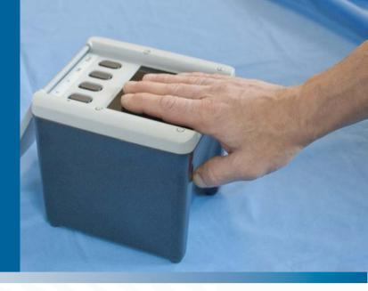
The **DS-30N** is a forensic quality fingerprint scanner manufactured as a separate optical unit driven by a backbone computer (including a notebook).
